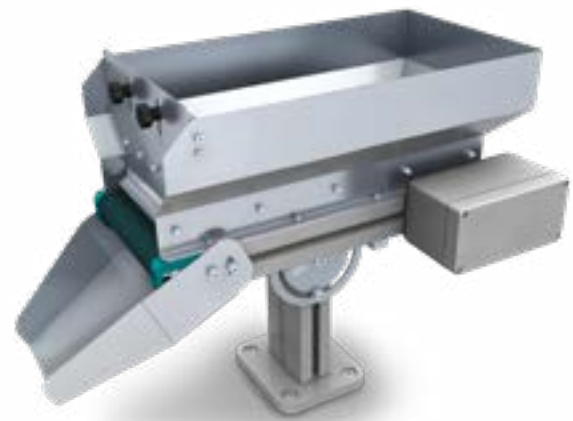
Figure: Custom design – hopper conveyor
